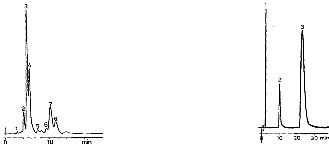
Fig. 7. Separation of hop acids in a beer extract. Peaks: 1 = \beta -acids; 2 = cis -isoadhumulone; 3 = cis -isocohumulone; 4 = cis -isohumulone; 5 = trans -isoadhumulone; 6 = \alpha -acids; 7 = trans -isocohumulone; 8 = trans -isohumulone. Mobile phase: hexane-diethyl ether (9:1); flow-rate 1.0 ml/min. Column: LiChrospher Si 100, 5 \mu m, 250 \times 3 mm, buffered with citric acid-sodium citrate, pH 2.6.
